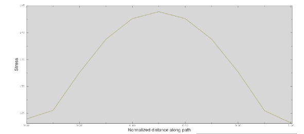
Figure 8: Hoop stress at Path3: through axial
